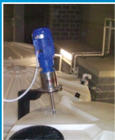
MIXQUIP STE series agitator mixing corrosive liquids... Titanium shaft and impellers.
